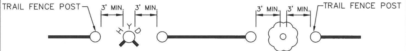
FENCE PLACEMENT AT TREES & FIRE HYDRANTS
