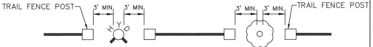
FENCE PLACEMENT AT TREES & FIRE HYDRANTS
